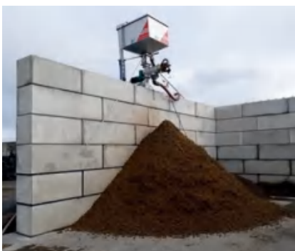
干物质含量为6.5%的粪污经过固液分离后干物质含量达到20%，分离能力为7 m 3 /h。 Raw material with 6,5 % dry matter is pressed to 20 % dry matter and reaches a throughput of 7 m 3 .
