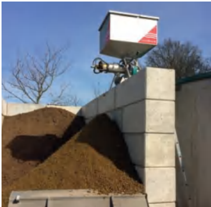
干物质含量为6.5%的粪污经过固液分离后干物质含量达到20%，分离能力为7 m 3 /h。 Raw material with 6,5 % dry matter is pressed to 20 % dry matter and reaches a throughput of 7 m 3 .
