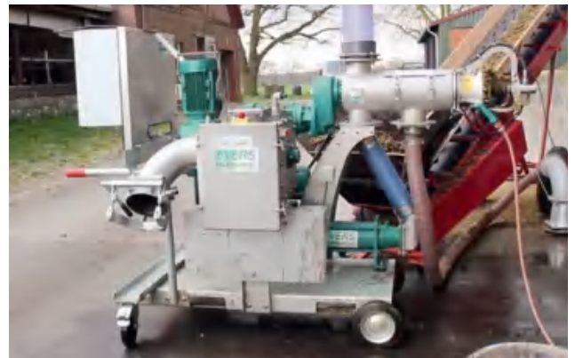
切割系统保护泵等技术为奶牛养殖生产有机垫料 | ComPress with integrated cutting system to protect pump and other technology produces organic bedding material for cow farming.
