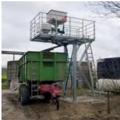
PSS 2.2-400 固液分离机在养猪场对干物质含量为5%的粪污进行分离，1.5天可以把拖车填满。 This PSS 2.2-400 with hopper runs on a pig production farm with a dry matter content of about 5% in the raw material. The tipping trailer is filled within 1,5 days.
