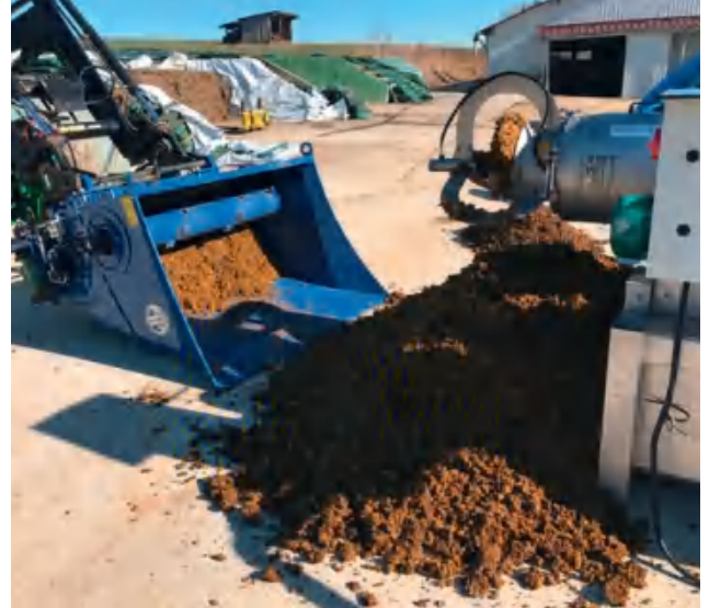
PSS 5.5-550 分离出的固体其干物质含量超过30% PSS 5.5-550 produces solids with more than 30% dry matter content as bedding material.
