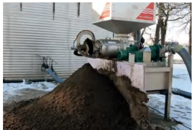
PSS 4-550 通过配套支架进行分离, 从而减少粪污的储存量 PSS 4-550 separates with extended pillars and releases the manure storage.
