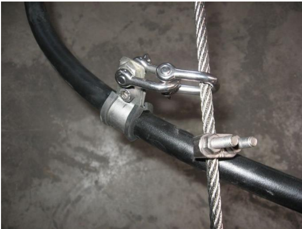
Fig. 4: Rope clip and 1st cable clamp
